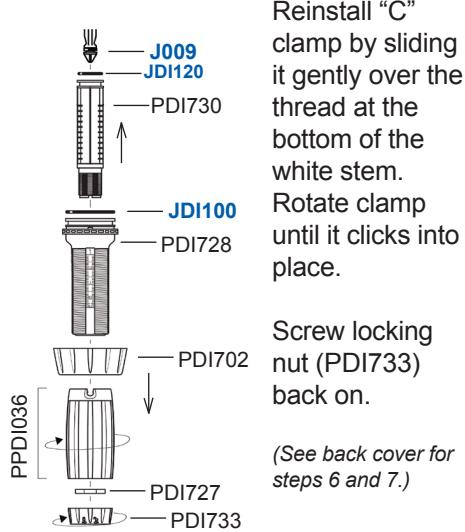
Reinstall "C" clamp by sliding it gently over the thread at the bottom of the white stem. Rotate clamp until it clicks into place.
