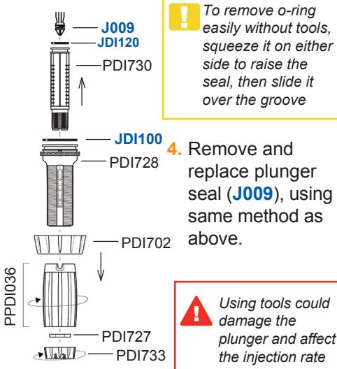
**!** To remove o-ring easily without tools, squeeze it on either side to raise the seal, then slide it over the groove
